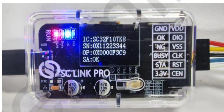
Fig. 2.2.3-2 SC LINK PRO S/N Offline Programming Completed
